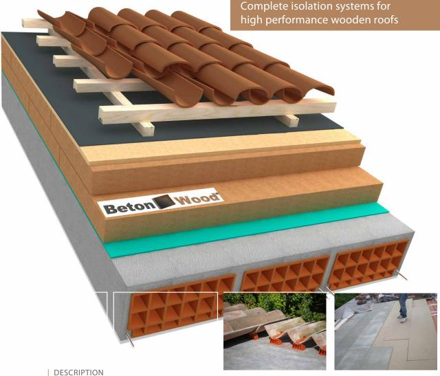
The complete natural insulating system for wood roof with high performances Roof SolutionD isorel is ideal for home wellness and comfort in all climatic zones.
