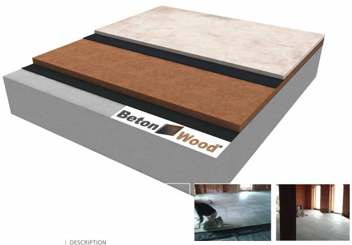
Complete dry building floor system on new and existing grounds which is composed by wood fiber panels with high density (250kg/m³) and excellent compression resistance (150 kPa) Fibertherm Base and BetonWood cement bonded particle boards with density 1350kg/m<sup>3</sup>.
