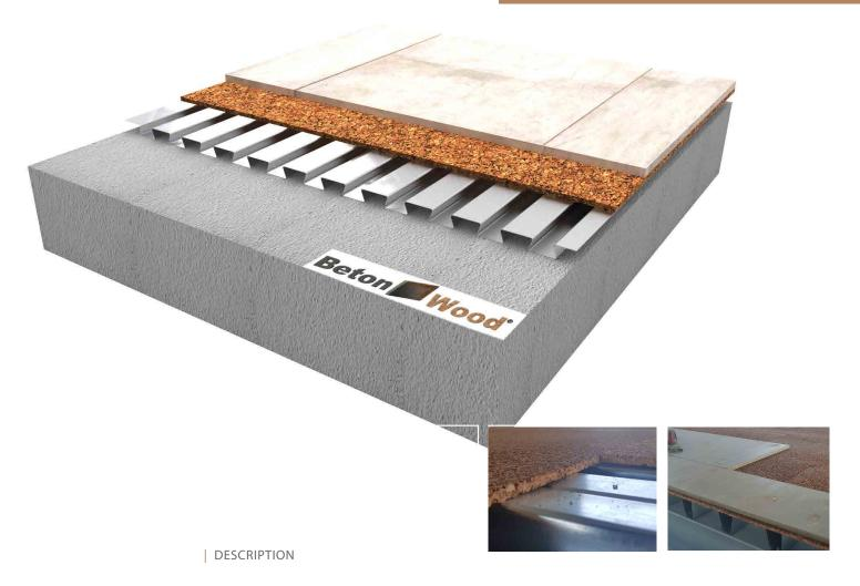
Complete system for dry floor supported by a dovetailed sheeting system. In this solution we'll have a layer of cement bonded particle boards BetonWood density 1350 kg/m³ and an insulating layer of super-compressed blond cork panels Cork Panels plus. Maximum durability over time is guaranteed, with international ETA certification.
