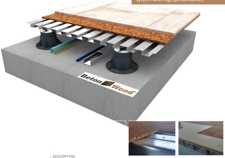
Complete system for elevated dry floor supported by a dovetailed sheeting system. In this solution we'll have a layer of cement bonded particle boards BetonWood density 1350 kg/m³ and an insulating layer of super-compressed blond cork panels Cork Panels plus. Maximum durability over time is guaranteed, with international ETA certification.
