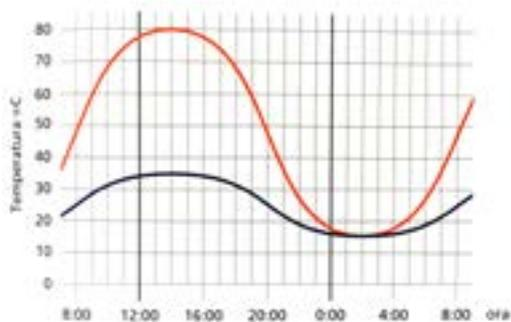
Temperature under the roof cover
